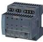
6EP1961-2BA51 SITOP PSE200U 3 A NEC CLASS 2 selectivity module 4-channel input: 24 V DC/12 A output: 24 V/4...
