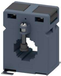
current transformer 250/1A, 5 VA CL 1.0
